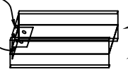
Back-to-back Base Cleat Connections with 2 M12 through bolts per bracket. DOUBLE COLUMN BASE CLEATS
